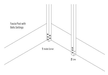
**STEP 1:** For structural support, ensure you have adequate framing behind the fascia, or the fascia is supported with sufficient blocking to exceed the minimum requirements for fascia post installation.
