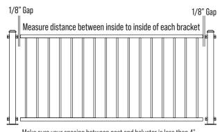
Make sure your spacing between post and baluster is less than 4"
