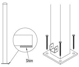
Fasteners to attach posts to deck or concrete
