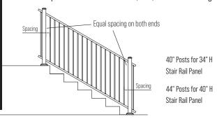
Check your local codes/ordinances for the proper spacing requirements from the bottom rail to the stairs as well as proper height requirements for the top rail.
