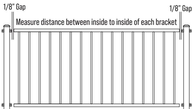
Make sure your spacing between post and baluster is less than 4"
