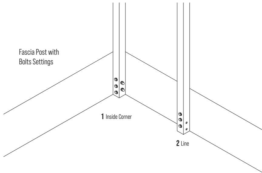
**STEP 1:** For structural support, ensure you have adequate framing behind the fascia, or the fascia is supported with sufficient blocking to exceed the minimum requirements for fascia post installation.
