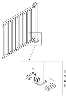
The post skirts do not need screws; the two halves will wedge together with a few gentle hits of a rubber mallet.
