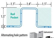
for #8 / #9 countersunk deck screws or 1/4 in. lag screws.
