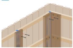
Finish the installation by adding 1x6 cover boards over the PostMaster posts.
